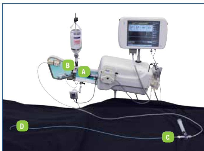
Figure 2: The CVi System showing points where pressure drops occur from the syringe to the catheter tip.
