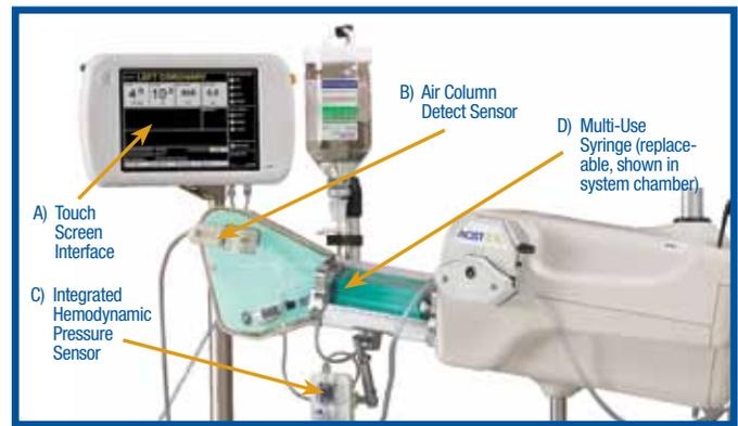
Figure 2. The ACIST CVI contrast injection system includes the Touch Screen Interface (A), the Air Column Detection Sensor (B), the Integrated Hemodynamic Pressure Sensor (C), and the Multi-Use Syringe (D), replaceable, shown in chamber.
